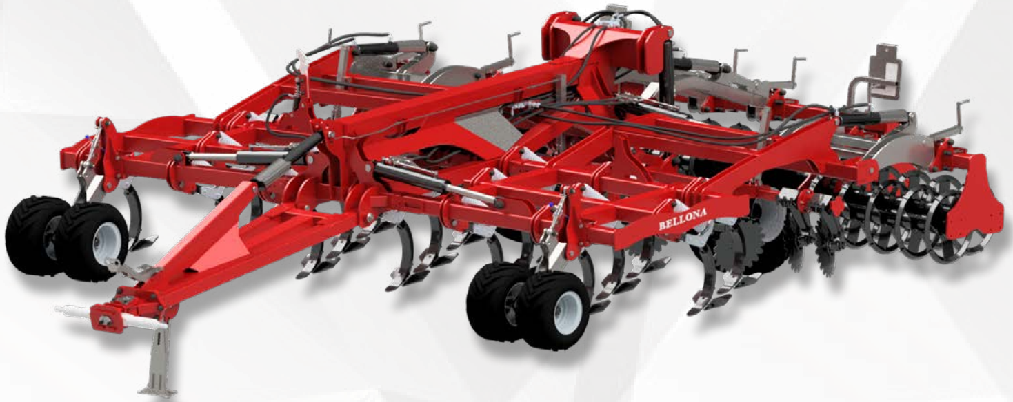
Front support wheels doubled
