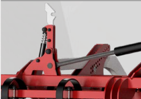
Hydraulic transport lock
