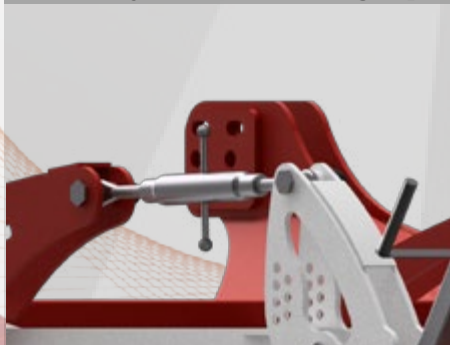
Manual adjustment of working depth
