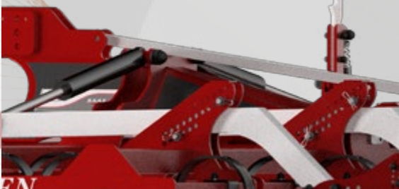
Manual adjustment of working depth
