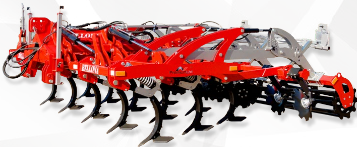
Spring-protected working element
