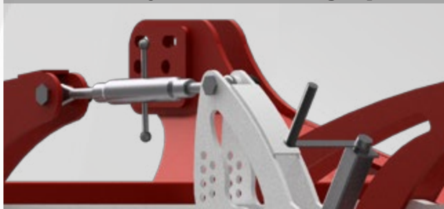
Manual adjustment of working depth
