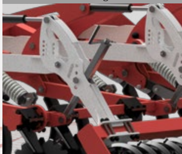
Independent adjustment of levelling discs
