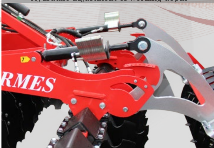
Hydraulic adjustment of working depth
